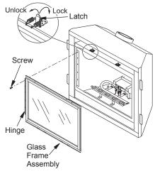
Figure 41 - Removing/Replacing Glass Door
